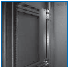
Hat sections positioned 19 inches on center to allow mounting of standard blank (CB series) panels for mounting electronic accessories
