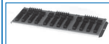
RPM-12 without Relays Installed
